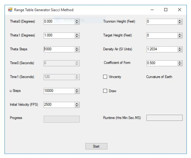
The rifle chosen to model is a 16-inch 50 caliber naval artillery gun for the Iowa class of fast battleships (BB-61 Iowa, BB-62 New Jersey, BB-63 Missouri, and BB-64 Wisconsin). 50 caliber means that the rifled barrel is  $50 \times 16$  inches in length = 800 inches = 66.667 feet. The following form is a comparison of the app's data with the range table found in Ordnance Pamphlet 770 © October 1941 by the Navy Department Bureau of Ordnance:
